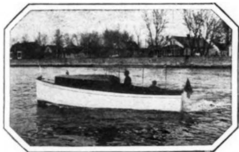
The motor of this tiny yacht is installed beneath the aft deck and exhausts through the open end of the boat. It can be attached or removed at will.
