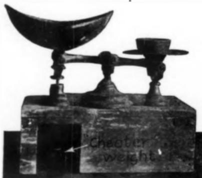
scales were mounted on a wooden box, as shown in the picture, and weighted from the bottom with padlocks, bolts, and other heavy objects. Another example of short
