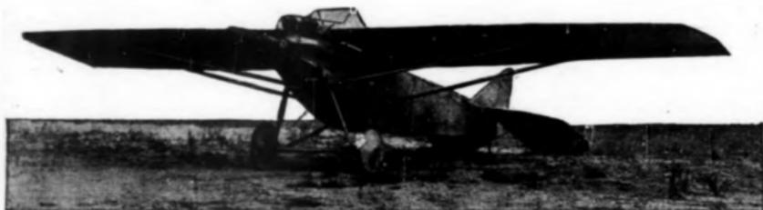
This little ship, weighing only 400 lbs., flies with a 20 horsepower motorcycle engine—and it doesn't use all the horsepower at that! For description of such a plane read accompanying article, the first ever written in non-technical language for the novice.
