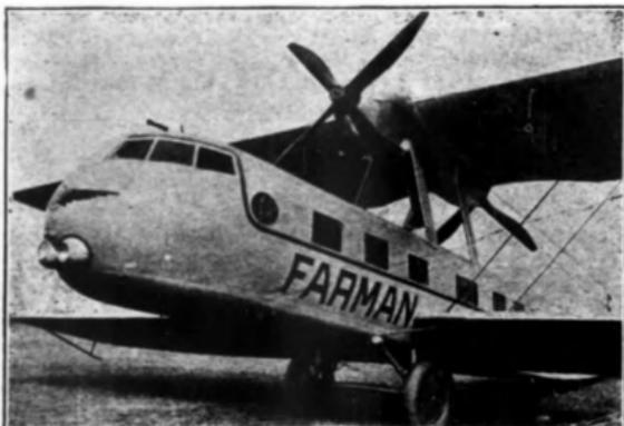
The interior of this new biplane accommodates 18 passengers and presents much the same appearance as a luxurious railway coach. The "bug eyes" in the streamline nose of the plane, shown above, are adjustable searchlights. Note the engine radiators incorporated in the struts anchoring the upper wing to the fuselage.
