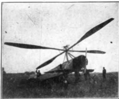
Four helicopter blades are intended to lift this machine into the air.
